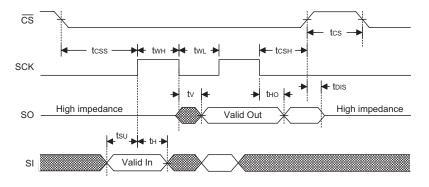
• Waveform 2 - Inactive clock polarity high
